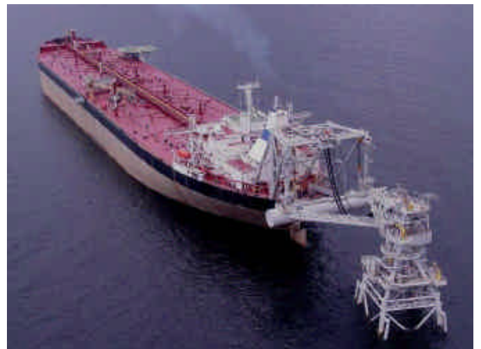
Figure 3D. The Floating Storage and Offloading vessel mated to its single point mooring structure.
